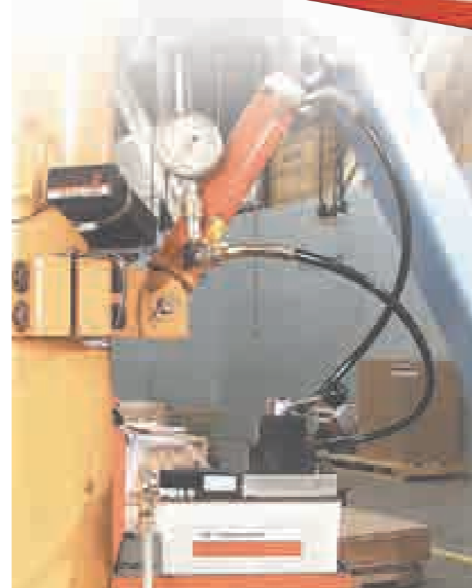
PA6D pump, DG100 digital pressure gauge and 25 ton cylinder used in a test fixture.
