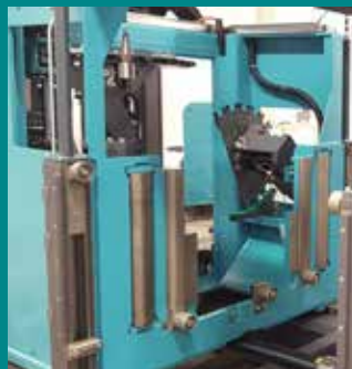
Robust clamping system and large tool changer.
