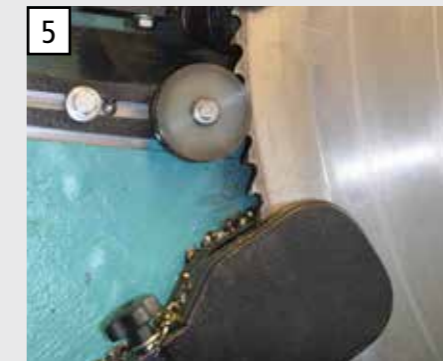
5 Chip remover cleans the saw blade for perfect cutting results and shorter cutting times.
