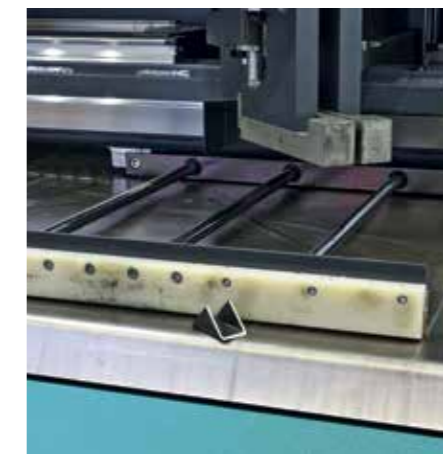
Integrated brush system for the removal of swarf, first cuts/residuals and gussets.
