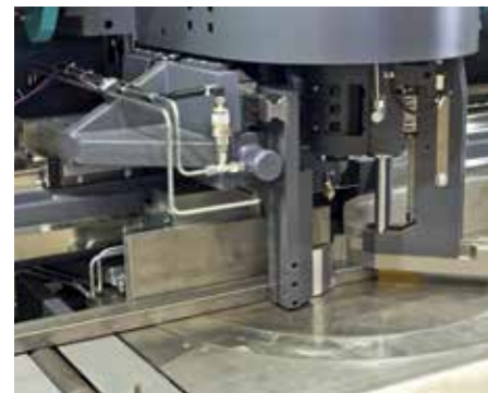
Swiveling vertical clamping device for mitre cuts for optimal material clamping and shortest remnant parts length (< 15 mm).
