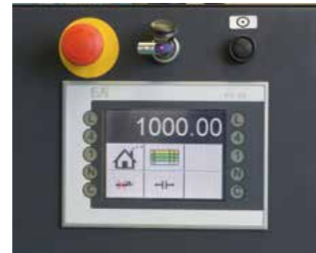
L 41 NC length measuring device (TL 450 only) Motor-driven adjustment of measurement length via NC control. The stop carriage is automatically clamped on reaching the position. Easy operation via touchscreen.
