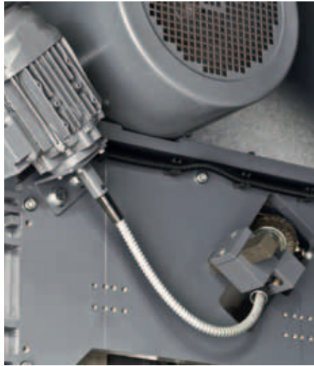
Swarf removal brush, reduced wearing level due to separate drive.
