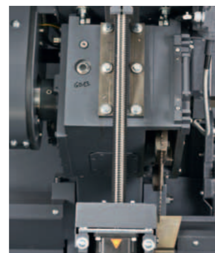
Saw blade feed with stable screw ball.
