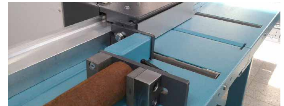
L 41 P automatic material infeed gripper and length stop Can be used as length stop or pusher plate.
