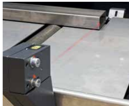
Laser light barrier for the cut identification.
