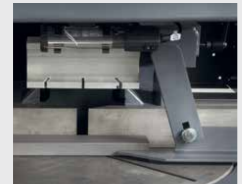
Horizontal clamping device on the removal side for material clamping during sawing.
