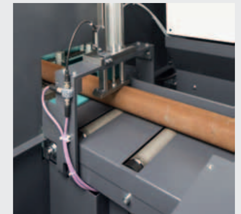
Automatic height measuring of materials and adjustment to the programmed values.
