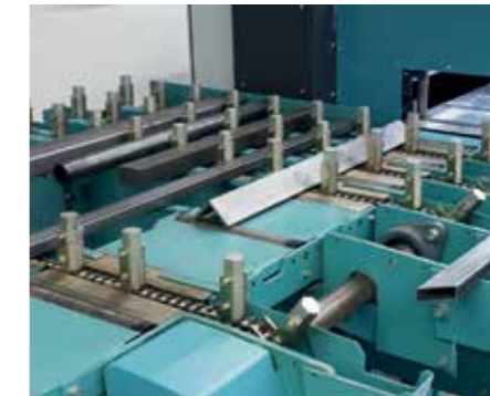
FM 1 flat magazine (SKL 450 NA only) For pre-storage of round and square material and profiles (including special profiles).
