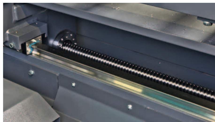
Highly precise cuts by positioning the automatic dispenser over the screw ball and servo motor.
