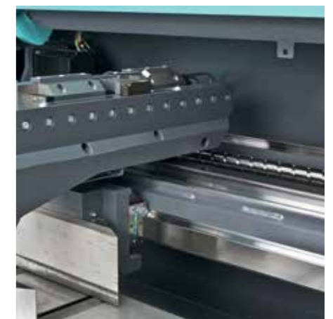
Highly precise positioning of the material via ball screw with brush-less servo motors. Guiding of the supply carriage on robust, maintenance free linear bearings.
