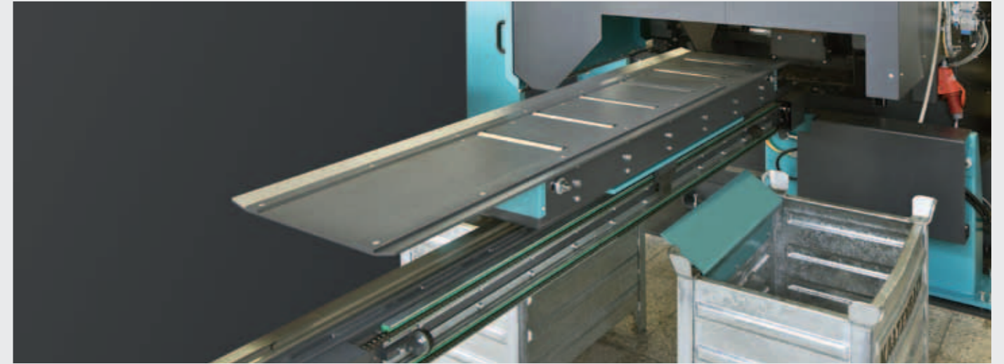
Extendible tipping roll rail, sorting positions can be selected freely.
