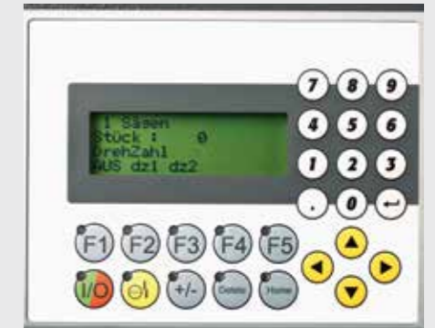
Control panel with illuminated text display (SKL H only).
