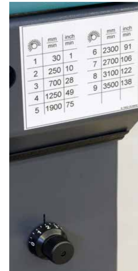
Feed regulator for universal, infinitely variable adjustment even during the sawing process.
