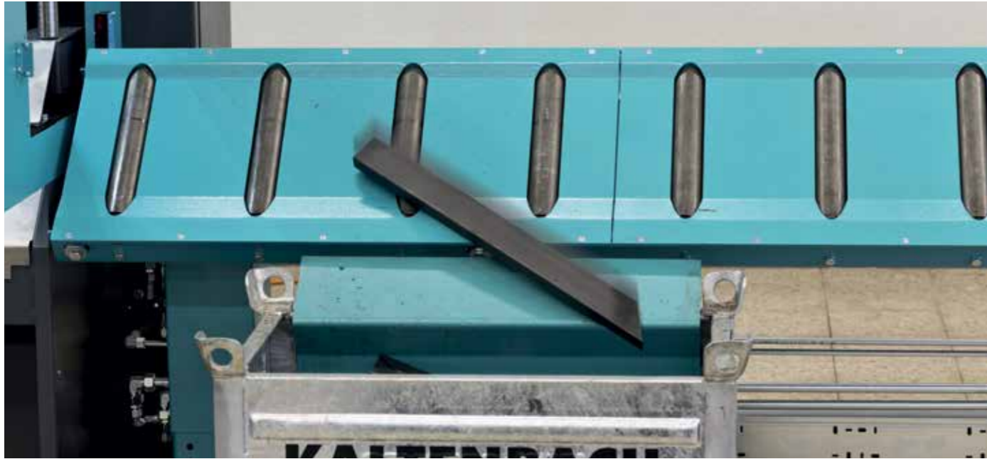
1 Tipping roll rail Sections can be adjusted flexibly to various positions via „teach in“.
