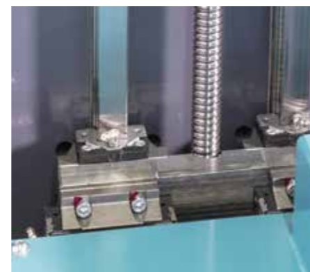
Faster, more precise drill carriage mounted on zero-play, pre-stressed linear guide elements. Ball screw with servomotor for high-precision positioning.
