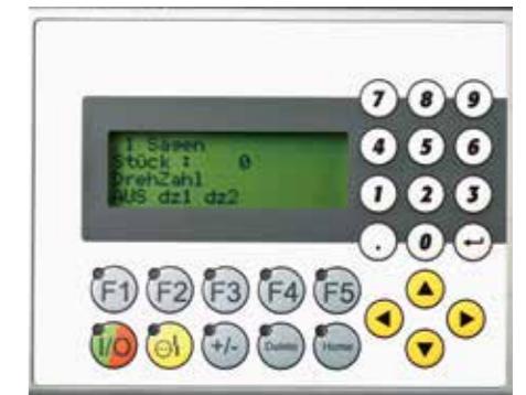
Input and diagnostic panel for the operating and programming.
