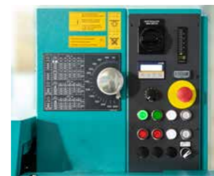
Easy and fast operation via push-button. Hydraulic saw blade feed, infinitely variable according to table.
