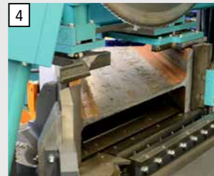
4 Automatic cross-section measurement during clamping for high process reliability.
