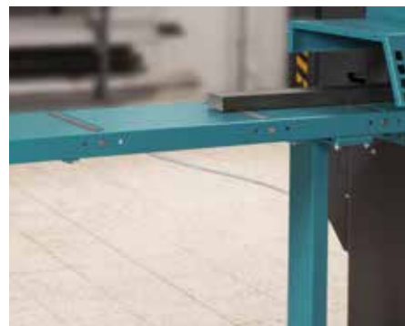
T3 feed conveyor Robust design, extendable by 1,000 mm.
