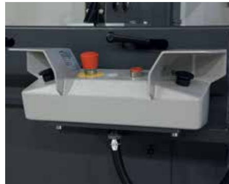
Two-handed operation instead of protection cover.
