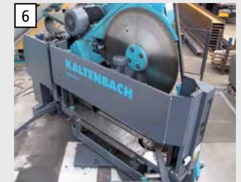
6 NC-controlled cutting angle setting for precise positioning.
