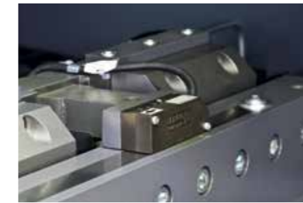
Material width measuring with automatic length correction for precise mitre cuts.
