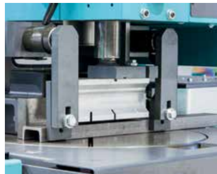
Horizontal clamping device on the right and/or left of the saw blade (option).
