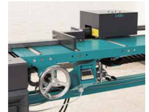
L 45 I length measurement device The stop is moved using a handwheel; the clamp is operated hydraulically by a hand valve. Digital length display.
