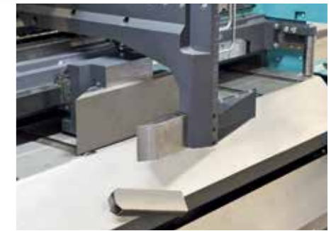
Offcut gripper for cut piece clamping during the saw cut, as well as for the sorting of offcuts/residual parts and good parts to pre-adjustable positions.
