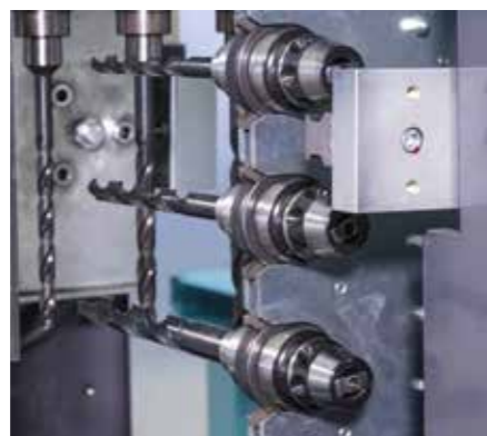
Each axis can be optionally equipped with three tools.
