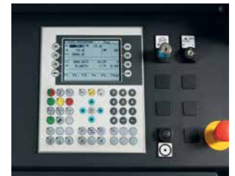
Simple operation and programming via NC control with input panel.
