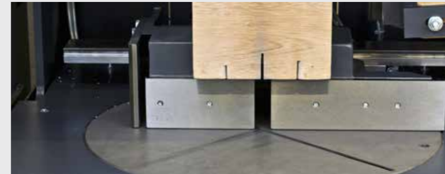
Rotary table for mitre cuts with a pivoting range of 180°.
