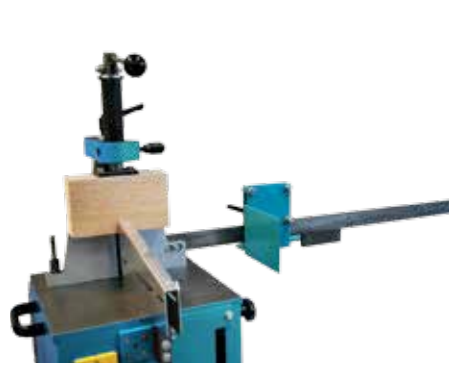
L10 length stop Working range 0 - 1000 mm.
