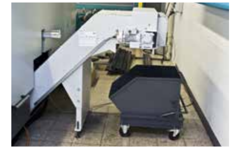
Slat-band chain conveyor for the automatic removal of swarf, cuts/remnants and gussets.
