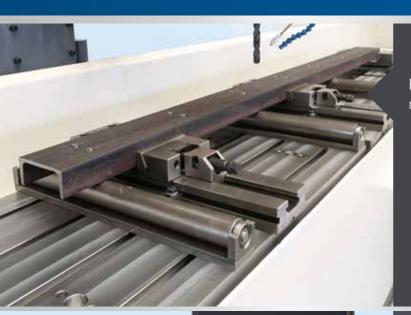
BAUER offers roller blocks to facilitate the movement of long workpieces.
