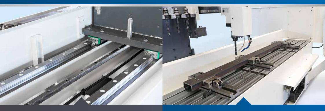
Largely dimensioned linear guides, large guide distance, feed x-axis through ground helical toothed rack, servo gear and servo motor.
