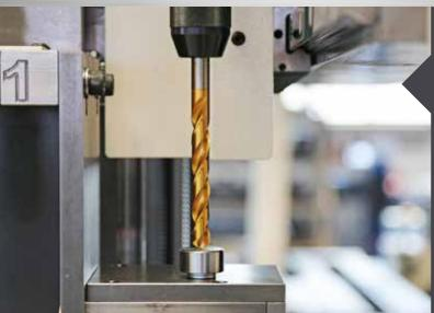
Automatic tool length measurement, movable swarf & splash water protection.
